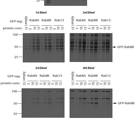
HeLa Flp-in Trex cells stably expressing GFP-empty, GFP-Rab8A, GFP-Rab8B and GFP-Rab13 were induced by Doxycycline ( $0.1\mu g/ml$ ) for 24h. The indicated protein extracts were subjected to SDS-PAGE analysis before transferred to nitrocellulose membrane and immunoblotted with Anti-GFP antibody or anti-Rab8B antibodies (bleed 1-4) overnight. Binding of the primary antibody was detected using anti-sheep (1:10,000) and visualised with ECL.
